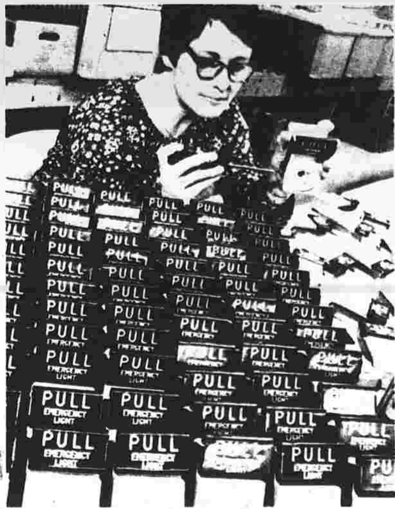
Emergency lights for military transport aircraft are assembled by Faye Hammaker at Midland-Ross Corp.'s Grimes Division Plant in Urbana, Ohio. Grimes manufactures electronic and mechanical lighting systems and controls and galley products for aerospace and other segments of the transportation industry. (UPI photo)
